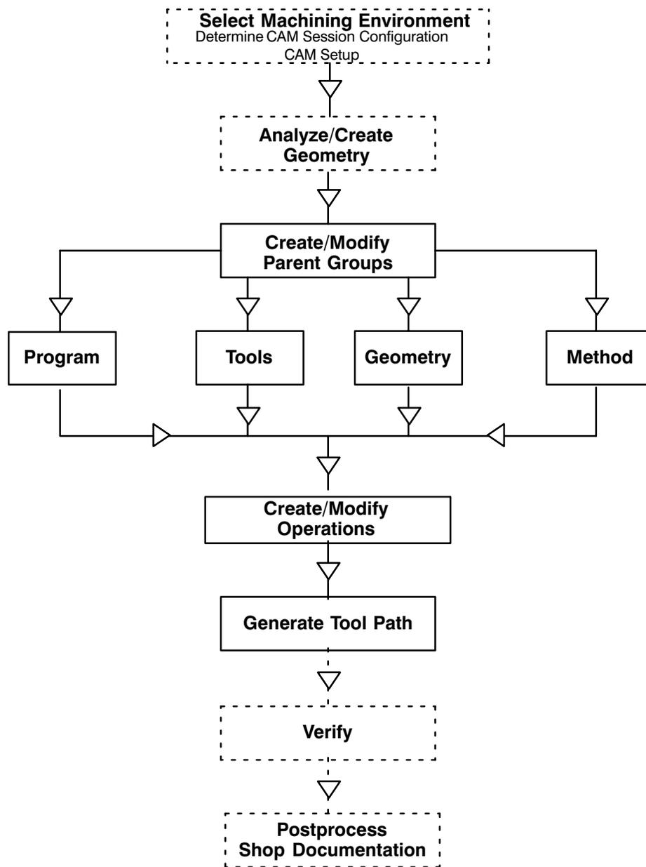
In this section of the workbook, you will create a Z-Level operation to cut all of the steep areas of the cover. You will define the geometry using a MILL\_AREA geometry parent group, generate a Z-Level Profile operation and then verify the results.
