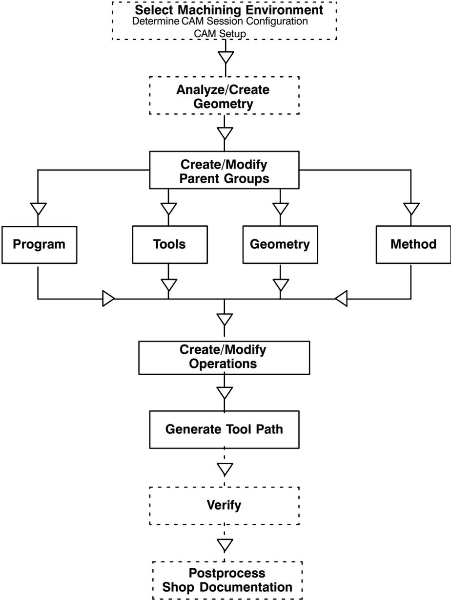
In this section of the workbook, you will create the drill geometry parent group and the drilling operations to spot drill and drill all holes.
