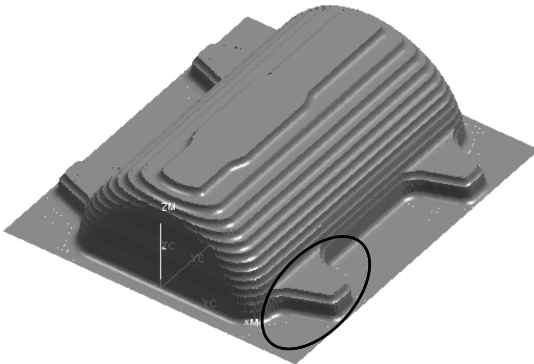
**Step 2** Modify the existing Cavity Milling operation to add a cut level at the top of the hold down pads. You will want to remove as much excess material as possible in the roughing operation.
