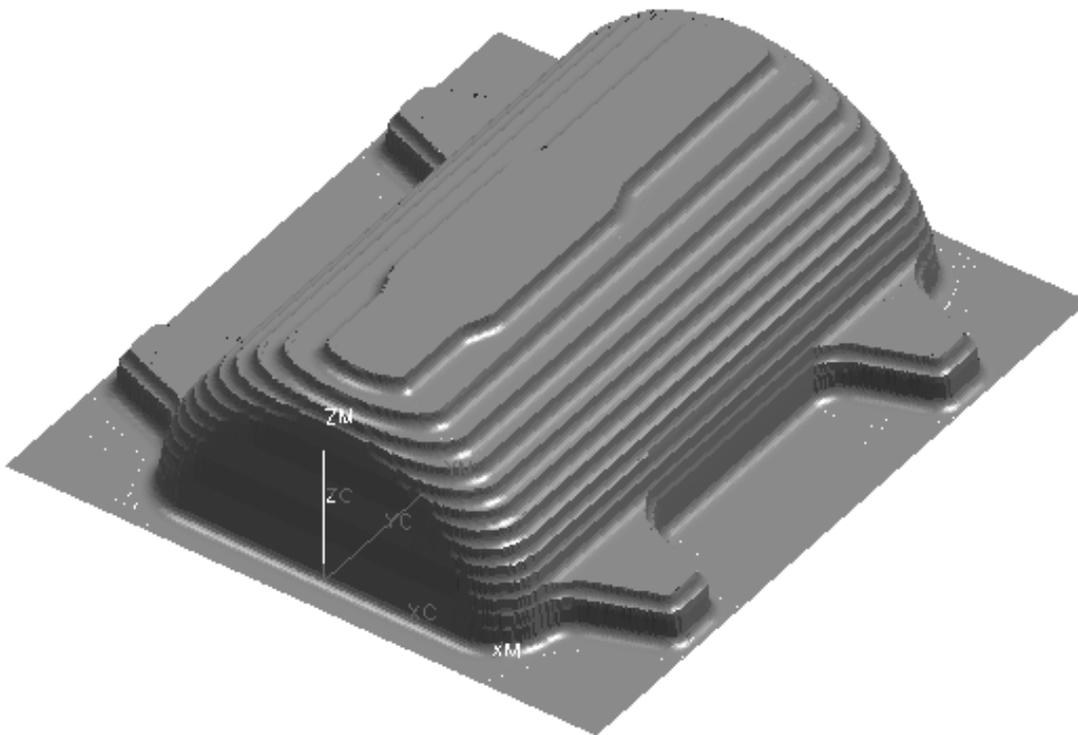
**Step 2** Create a MILL\_AREA geometry parent group that describes the area for Z-Level machining.
