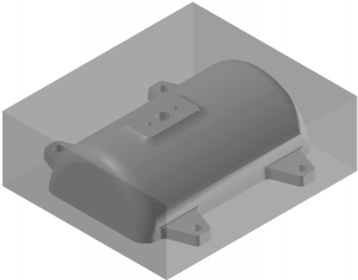
**Step 8** Create/Assign the Geometry Parent Group necessary for the Cavity Milling operation that you will be creating.
