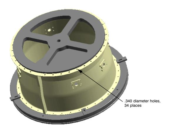
Step 8 Create the operations necessary to spot-drill, drill and ream the 34 holes located on the top flange.
