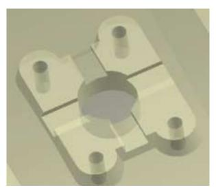
Use tool EM\_.250x.03 and verify your results. Use the looping technique of Sequential Mill to rough the dovetail slot.
