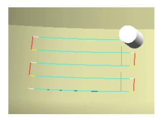
Step 4 Create a Sequential Milling operation to machine the outer periphery of the manifold flange.
