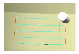
Step 4 Create a Variable Contour operation to machine the outer periphery of the manifold flange.
