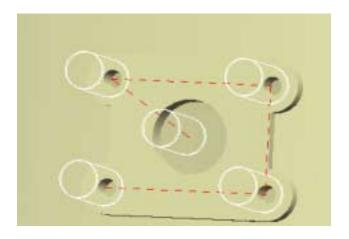
Step 6 Create a Variable Contour tool path to machine the dovetail slots.
