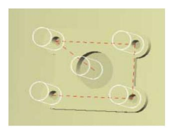
Step 6 Create a Sequential Milling tool path to machine the dovetail slots.
