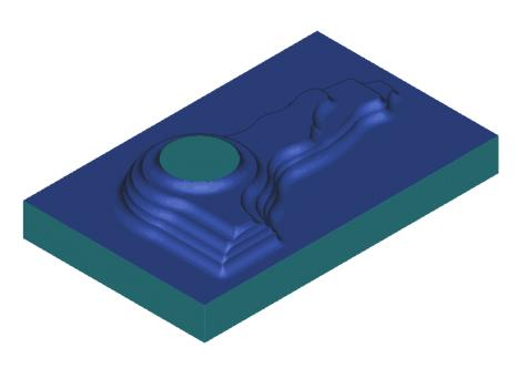
In Process Model from previous Cavity Mill Operation
