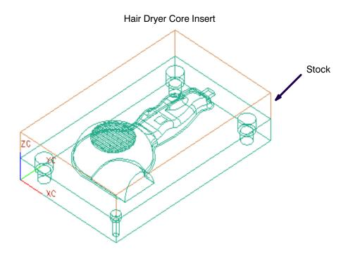
There is one Cavity Milling, six Z-Level and eleven different Fixed Contour operation subtypes under the Mill Contour Set-up. Each operation subtype represents a different method of material removal. Selection of the operation subtype is normally based on cutting tool availability, machine rigidity, type of material being cut, geometry or feature configuration, speeds and feeds and desired finish.
