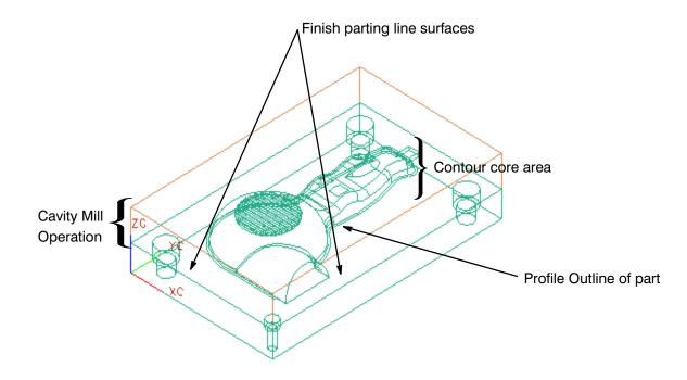
**Step 4** Examine the various **Method** parent groups. Methods are based on machining practices such as rough or finish. Assign options as required.
