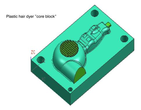
You will begin this project by using the provided Process Plan which will guide you through the various steps required to machine the core block.
